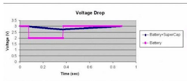
Fig. 3. Voltage drop of battery alone vs. battery plus supercapacitor.
