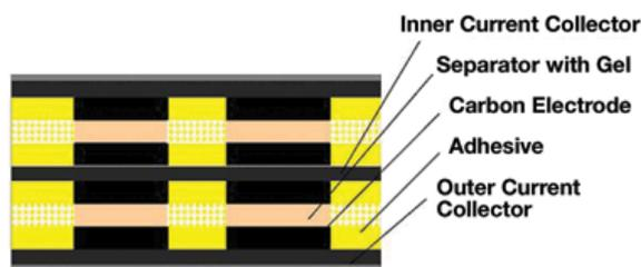
Example for 2 layer wafer - 1.4V capacitor
