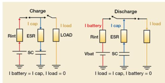
*Fig. 1. Battery-powered pulse circuit.*
